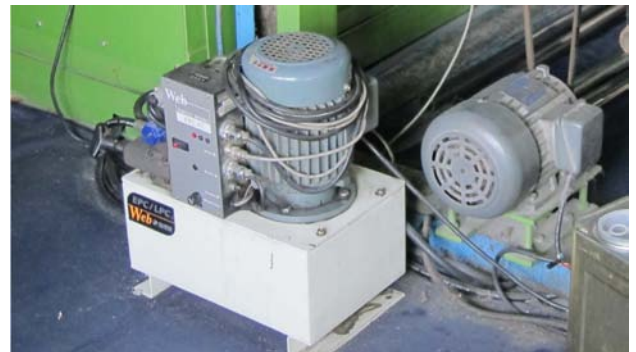
Controller Series 67 is installed on TOUGU DENKI Hydraulic Actuator directly
